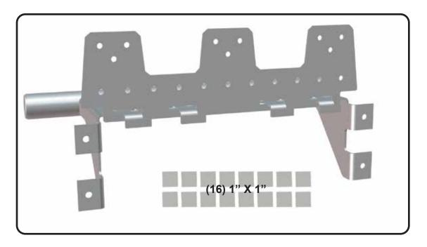
Identify the (12) minimum required holes that you need to use when installing the LedgeLock. However, if you need to adjust the holes that you use according to the studs in the roof, do so. Make sure that you use a minimum of (12) holes evenly distributed over the LedgeLock.
