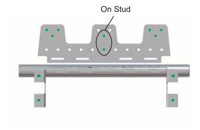
Recommended Wood Anchorage Bolt Pattern (Minimum 8 bolts required in Roof Plate)
